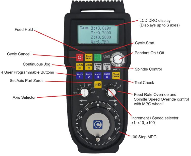
Take the control to where the work is! A game changing tool, the Centroid Wireless MPG Control Pendant allows the operator to conveniently and precisely set up jobs and tools remotely.
