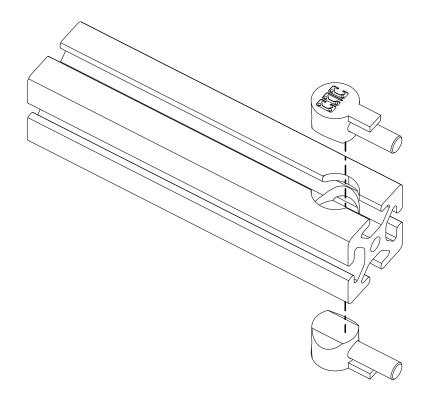
• Slide the anchors into the cable track extrusion as indicated.
