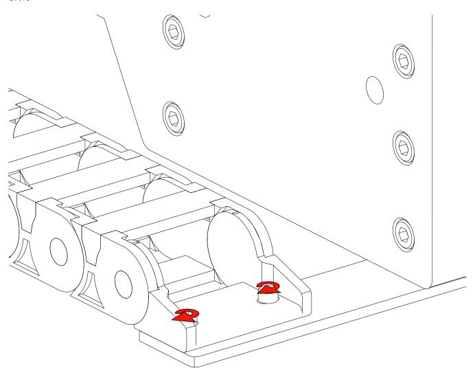
• Tighten the fixed end to the lower bracket.
