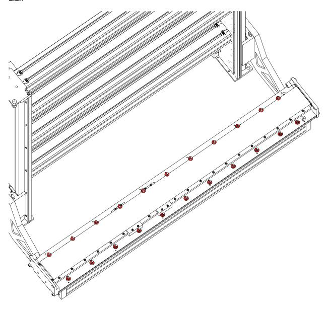
• Tighten the gantry axis bolts.
