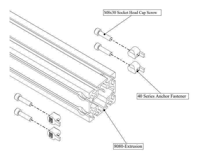
• Insert socket head cap screws into anchor fasteners as indicated.
