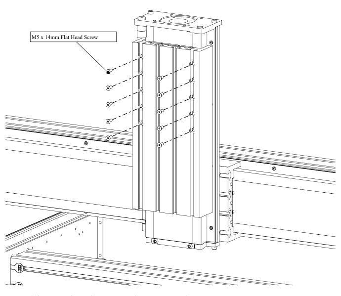
• Attach the moving plate to the Z axis using the screws removed in previous steps.
