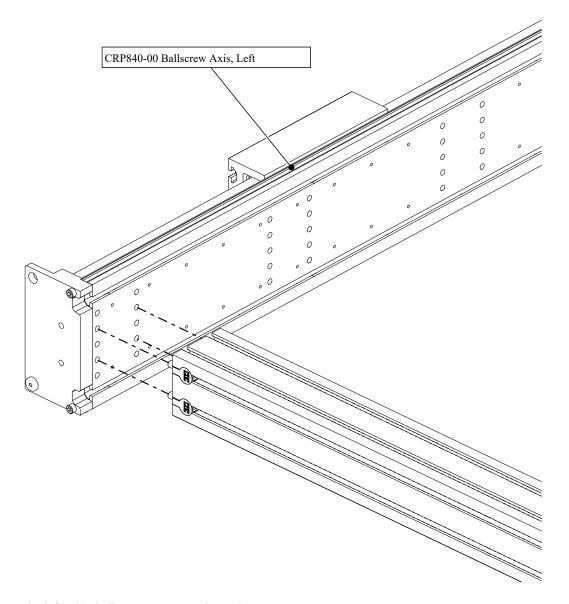
• Thread the screws into the left table ballscrew axis as indicated.
