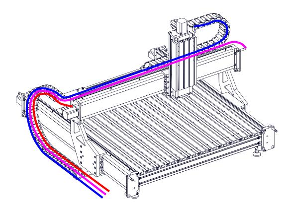
• Route the indicated sensor cables as shown (see table on next page). The remaining three sensor cables can be routed directly to your control box without going through cable track.
