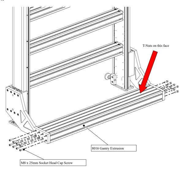
• Attach gantry extrusion to the risers with the M8 x 25mm fasteners.
