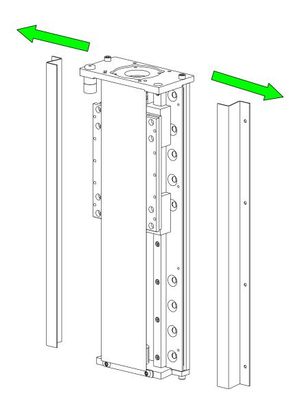
• Remove the metal dust covers from the Z-Axis.
