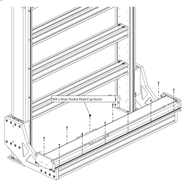
• Attach the metal dust covers using the screws removed in previous steps.
