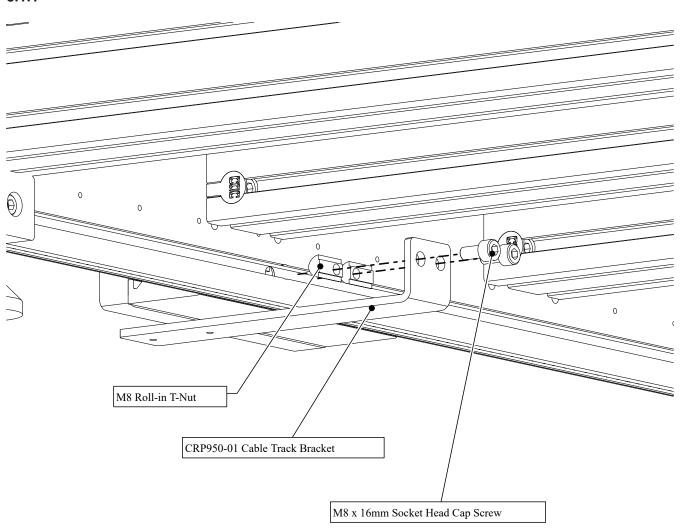
• Install the lower cable track bracket onto the bottom of the base of the machine.
