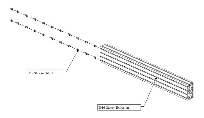
• Slide t-nuts into gantry extrusion.
