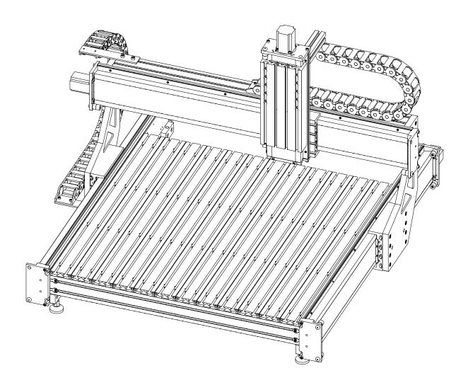
• Repeat the previous steps to install the remaining tabletop extrusion pieces.
