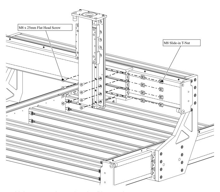
• Slide the M8 T-Nuts into the gantry plate and install the Z-axis to the gantry.
