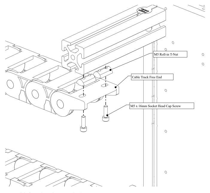
• Install the free end onto the extrusion bracket.
