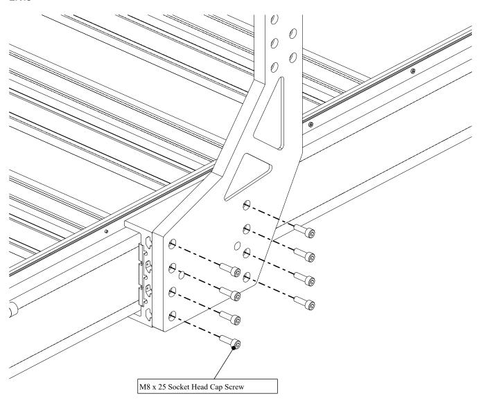
• Thread socket head cap screws into the T-Nuts.
