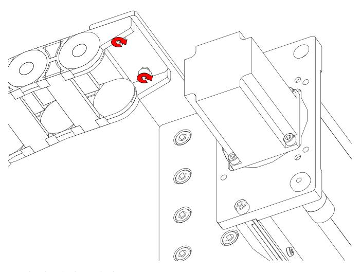
• Tighten the end to the upper bracket.
