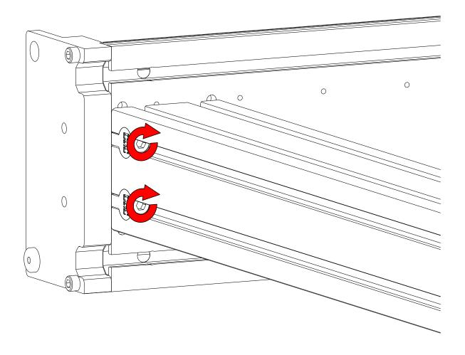
• Tighten the indicated fasteners
