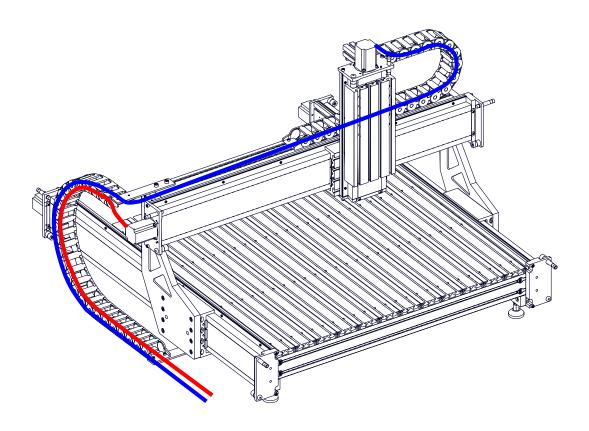
• Route the indicated motor cables as shown. The remaining two motor cables can be routed directly to your control box without going through cable track.
