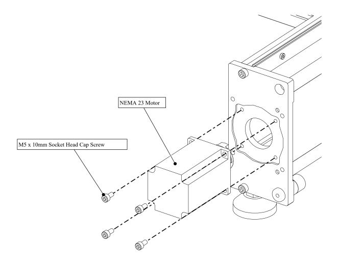
• Attach the motor to one of the table axes as indicated.
