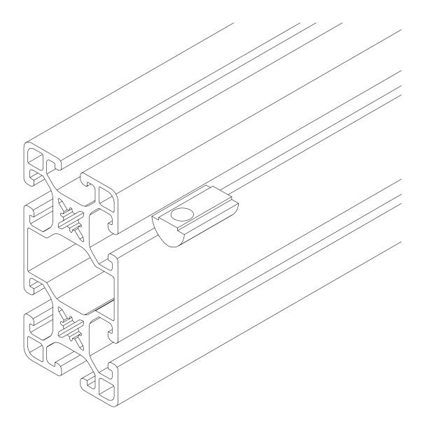
• To install in the appropriate extrusion slot, position the T-Nut as indicated.
