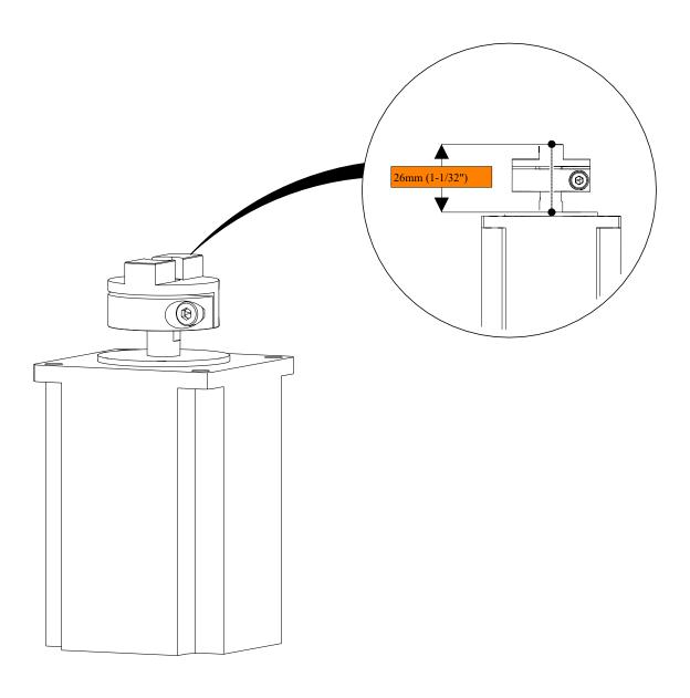
• Position the end of the coupler 26mm (1-1/32") from the motor flat.
