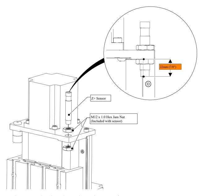
• Install sensors as indicated at each sensor location (see step 7.1.2).
