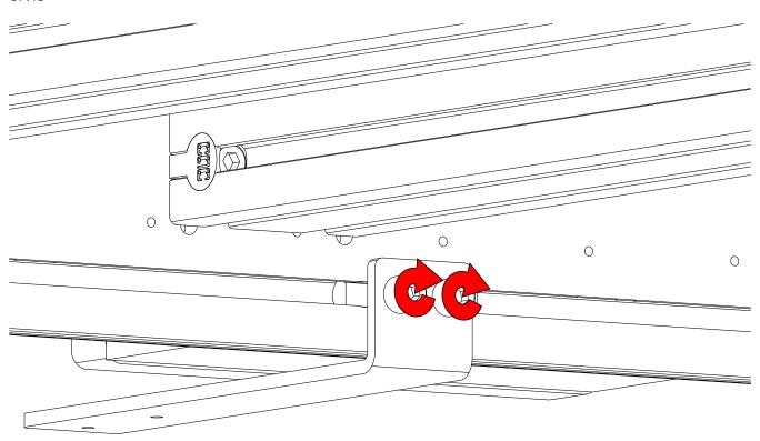
• Tighten the indicated fasteners.
