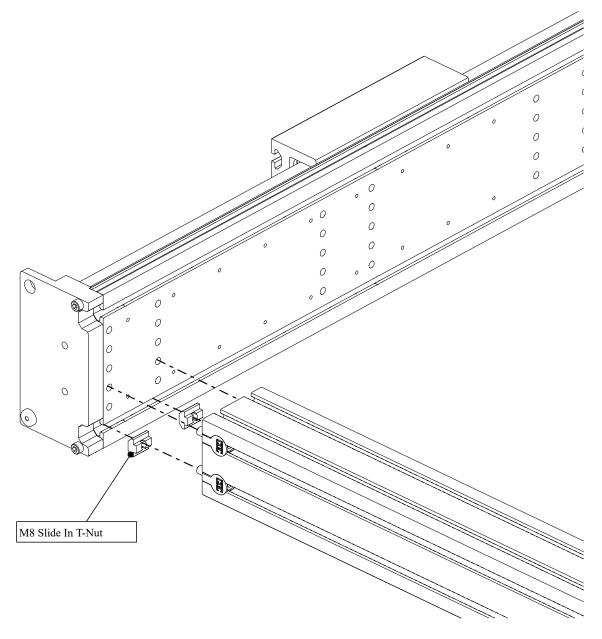
• Alternately, you can use the provided slide-in t-nuts to lower the crossmember extrusion.
