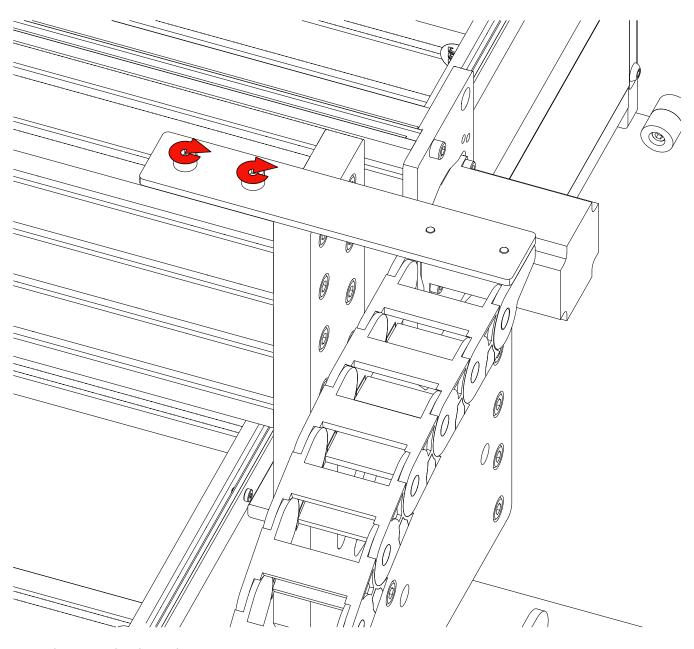
• Tighten upper bracket to the gantry extrusion.
