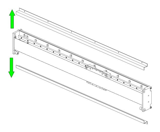
• Remove the metal dust covers from the gantry axis.
