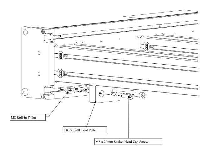
• Attach a foot plate to a ballscrew axis as indicated.
