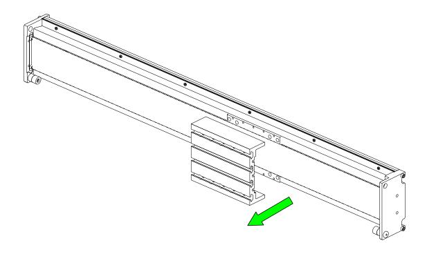
• Remove the moving plate and set aside.
