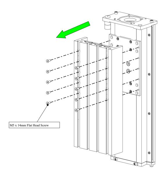
• Remove the moving plate from the Z axis.
