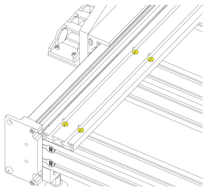
• Partially tighten the tabletop extrusion fasteners.
