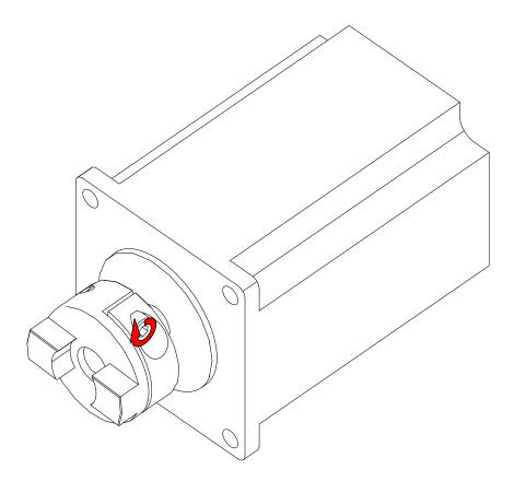
• Tighten the clamp bolt as indicated.
