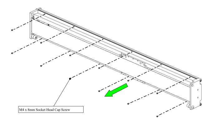
• Remove the metal dust cover screws from the gantry axis and set them aside.
