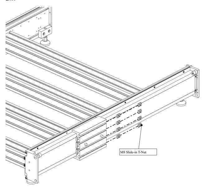
• Slide slide-in T-Nuts onto the right table axis as indicated.
