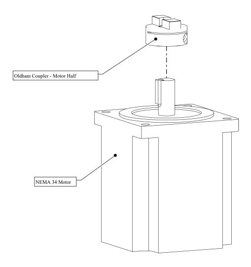
• Slide the motor side of the oldham coupler onto the motor as indicated.
