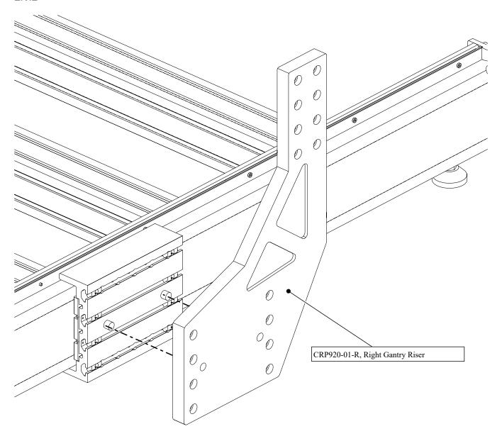
• Attach the right gantry riser to the extrusion.
