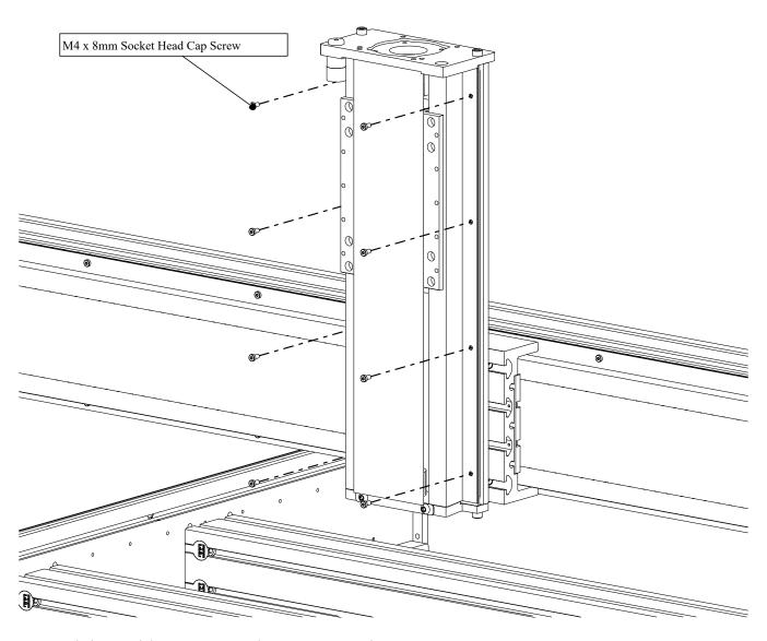
• Attach the metal dust covers using the screws removed in previous steps.
