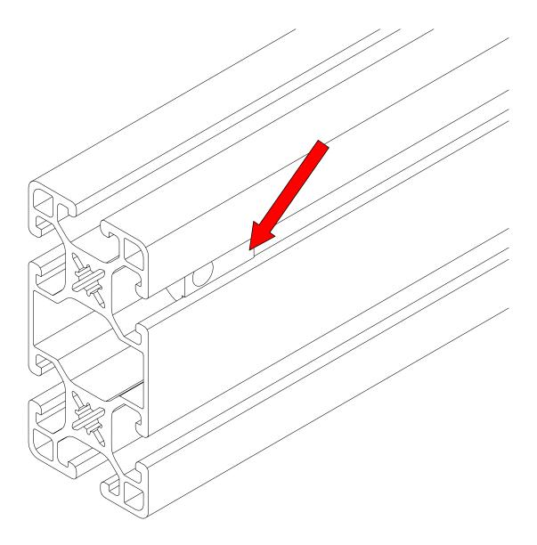
• When properly installed, the indicated face of the T-Nut will be parallel with the face of the extrusion.
