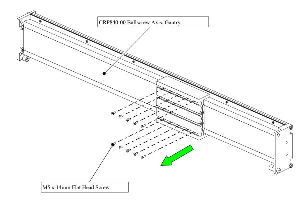
• Remove the indicated screws holding the moving plate to the gantry ballscrew axis.
