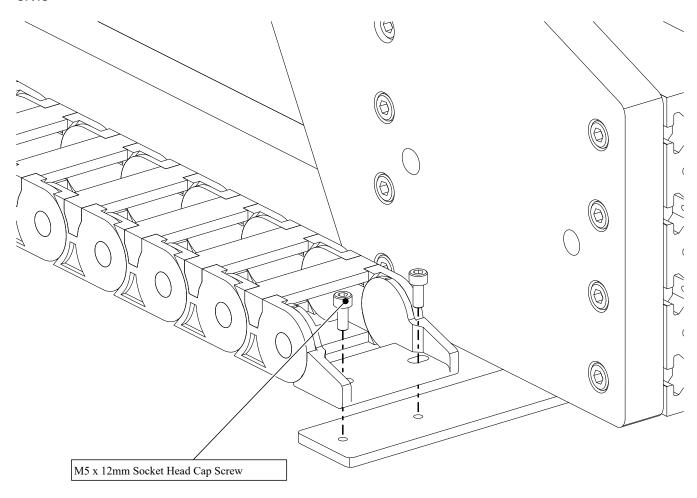
• Attach the fixed end of the cable track to the bracket as indicated.
