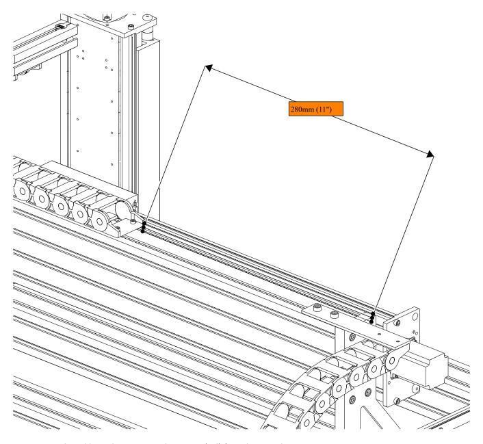
• Position the cable track approximately 280mm (11") from the riser plate.
