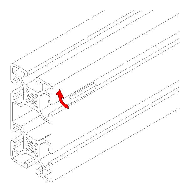
• Insert the T-Nut into the extrusion slot and rotate 90°.
