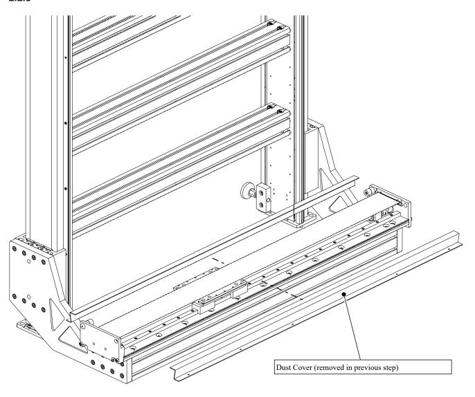
• Slide the metal dust covers back on the gantry axis as indicated.
