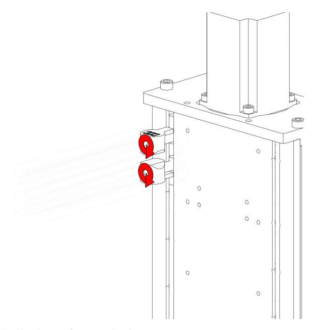
• Tighten the cable track extrusion fasteners as indicated.
