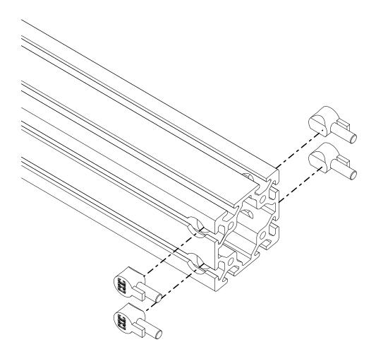
• Slide the anchor fasteners and screws into the extrusion counterbores.
