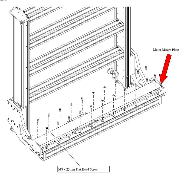
• Attach the gantry ballscrew axis to the gantry extrusion oriented with the motor mount plate on the indicated side.
