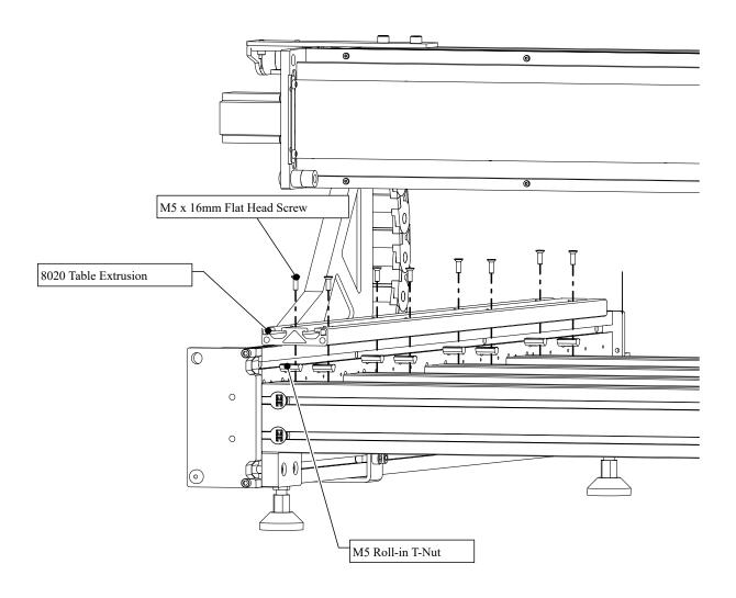
• Attach a piece of tabletop extrusion to the machine crossmembers as indicated.
