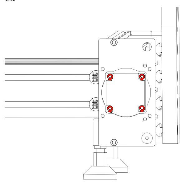
• Tighten the indicated fasteners.
