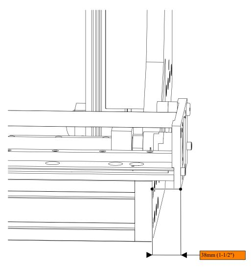
• Position the axis so the motor mount plate is 38mm (1-1/2") from the riser.
