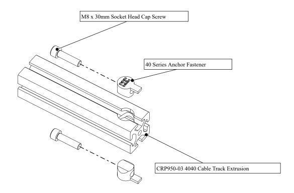
• Insert the M8 x 30mm bolts into the provided anchors and place the anchors in the bracket extrusion provided.
