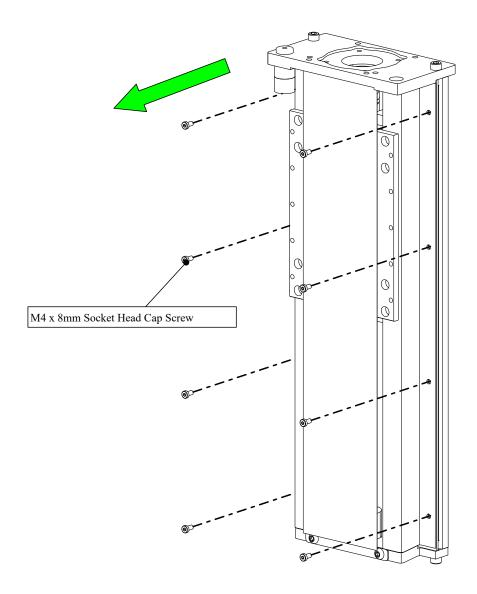
• Remove the metal dust cover screws from the Z axis and set them aside.
