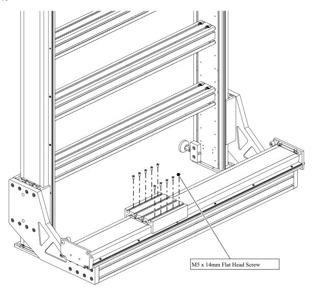
• Attach the moving plate to the gantry axis using the screws removed in previous steps.
