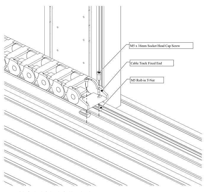
• Install the fixed end of a length of cable track to the gantry extrusion.
