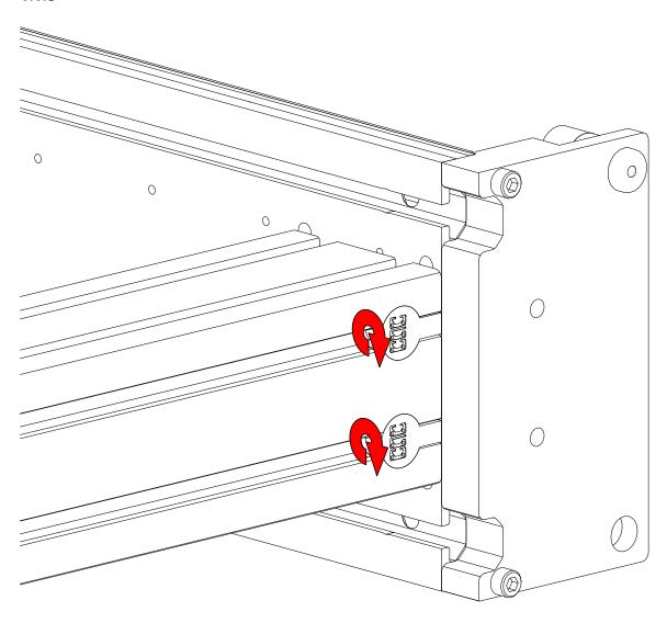
• Tighten all remaining crossmember anchor screws.
