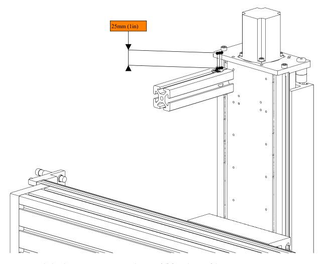
• Position the bracket extrusion approximately 25mm (1") from the top of the Z axis.
