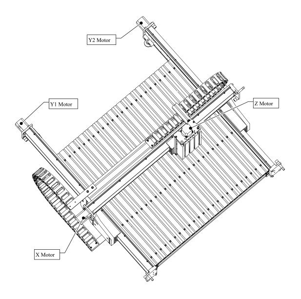
• Install motors on the remaining axes.
