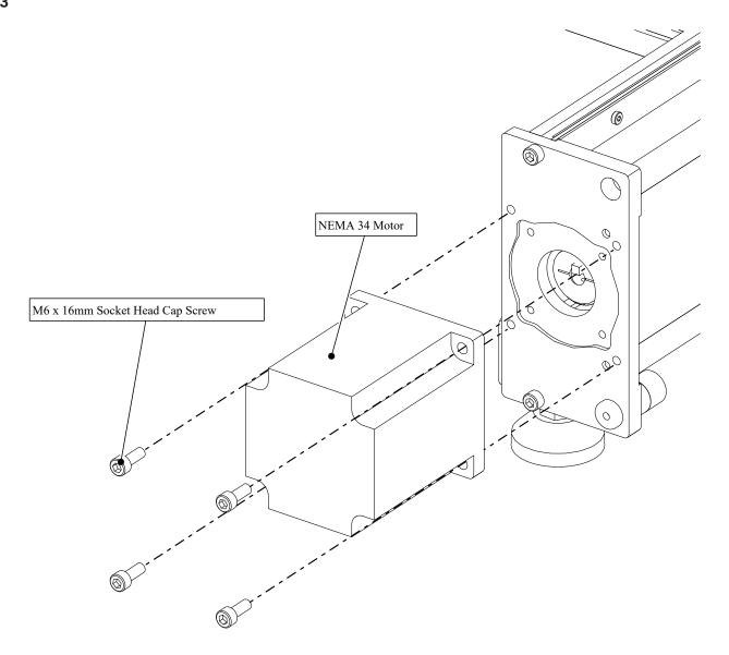
• Attach the motor to one of the table axes as indicated.
