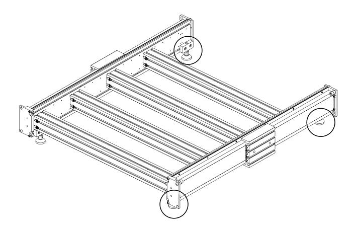
• Repeat this process to install the remaining leveling feet at the indicated locations.
