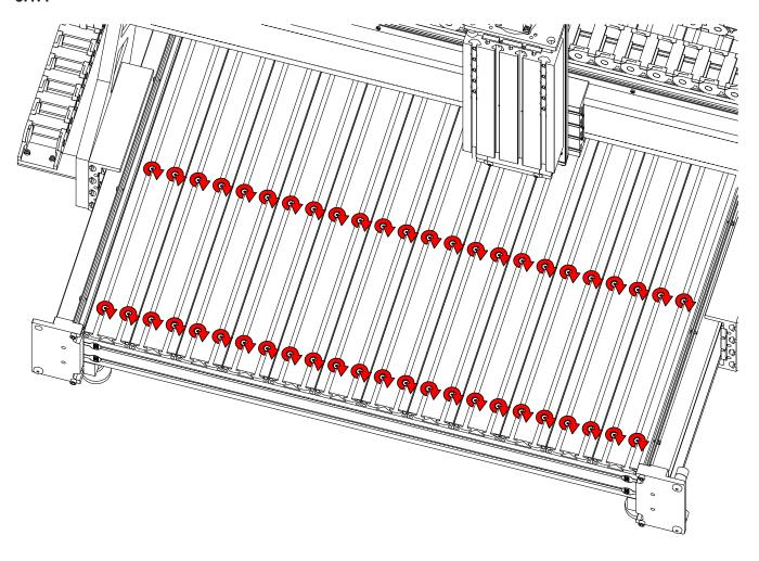
• Fully tighten the tabletop extrusion fasteners.
