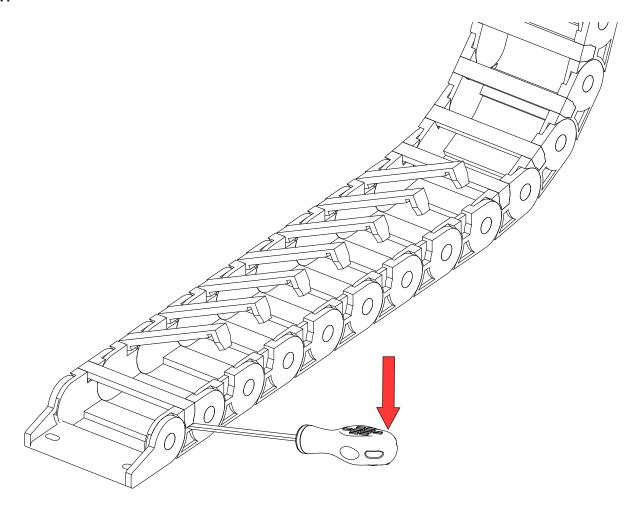
• To route cables through the cable track, use a screwdriver to lift open the individual cable track sections as indicated.
