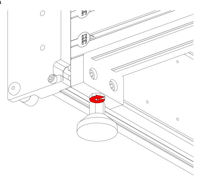
• Tighten the lock nut.
