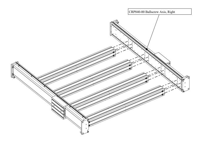
• Add anchor fasteners and screws to the other side of the extrusion and attach the right table ballscrew axis.
