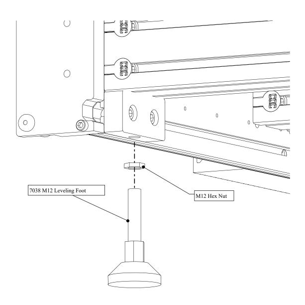
• Install the lock nut onto the leveling foot and thread the leveling foot into the foot plate.
