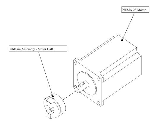
• Slide the motor side of the oldham coupler onto the motor as indicated.
