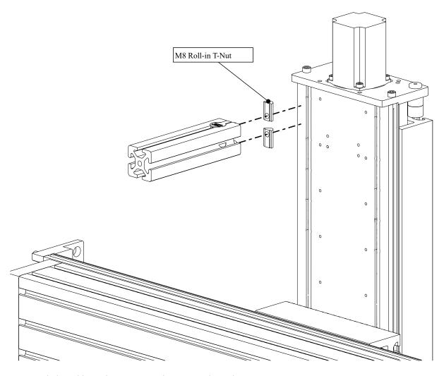
• Attach the cable track extrusion to the Z axis indicated.
