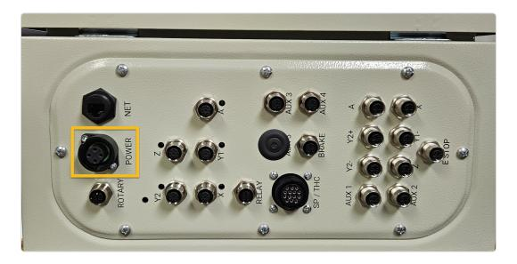
• Connect the RD-24 Power Cable to the Power port.
