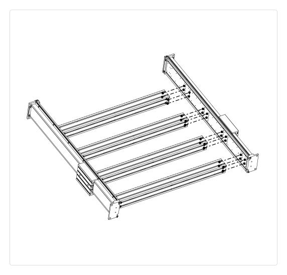
• Add anchor fasteners and screws to the other side of the extrusion and attach the right table ballscrew axis.
