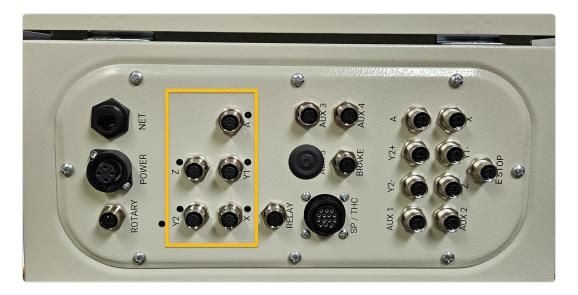
• Connect each motor control cable to the appropriate motor port.
