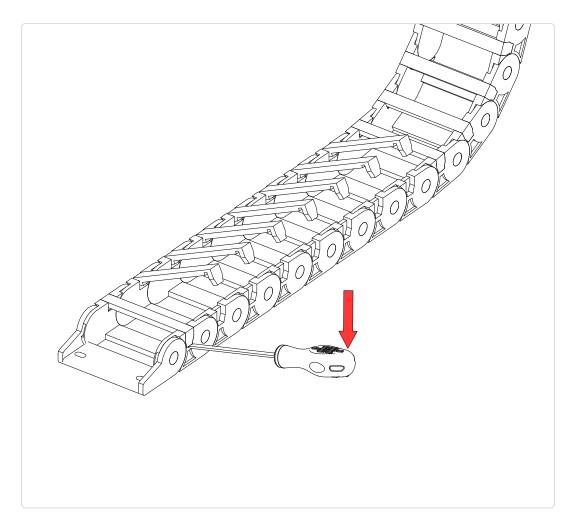
• To route cables through the cable track, use a screwdriver to lift open the individual cable track sections as indicated.
