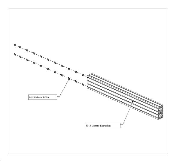
• Slide t-nuts into gantry extrusion.
