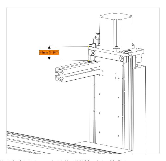
• Position the bracket extrusion approximately 44mm (1-3/4") from the top of the Z axis.
