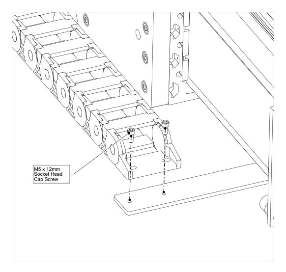
• Attach the fixed end of the cable track to the bracket as indicated.
