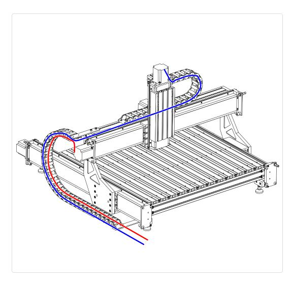
• Route the indicated motor cables as shown. The remaining two motor cables can be routed directly to your control box without going through cable track.
