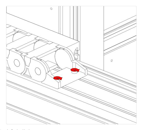
• Tighten the fixed end in place.
