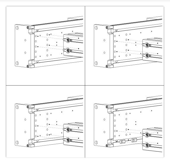
• Alternately, you can use the provided slide-in t-nuts to lower the crossmember extrusion.
