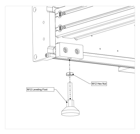
• Install the lock nut onto the leveling foot and thread the leveling foot into the foot plate.
