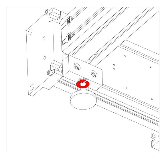
• Tighten the lock nut.
