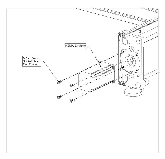
• Attach the motor to one of the table axes as indicated.
