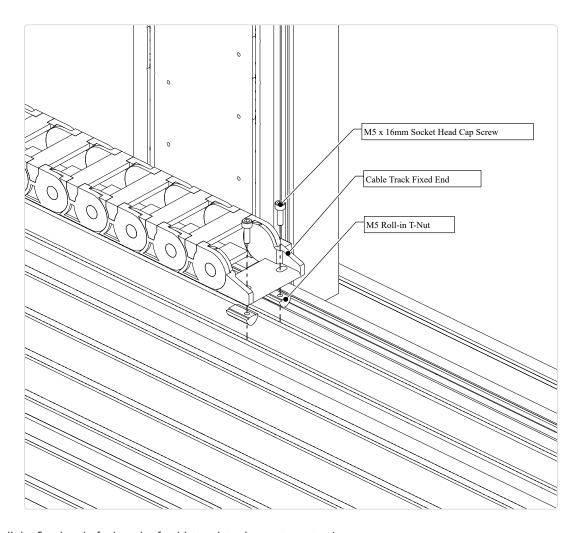
• Install the fixed end of a length of cable track to the gantry extrusion.
