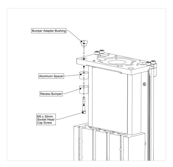
• Attach the Z axis bumper to the motor mount plate.
