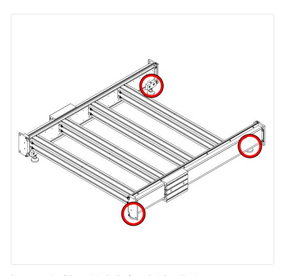
• Repeat this process to install the remaining leveling feet at the indicated locations.
