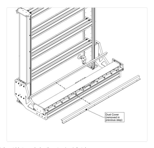
• Slide the metal dust covers back on the gantry axis as indicated.
