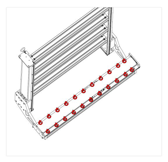
• Tighten the gantry axis bolts.
