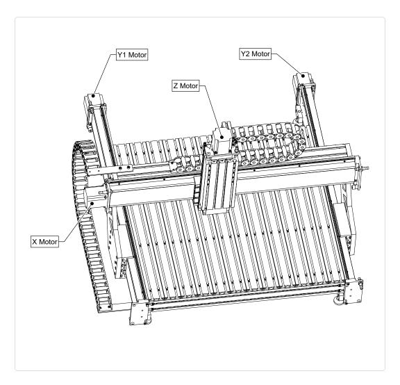
• Install motors on the remaining axes.
