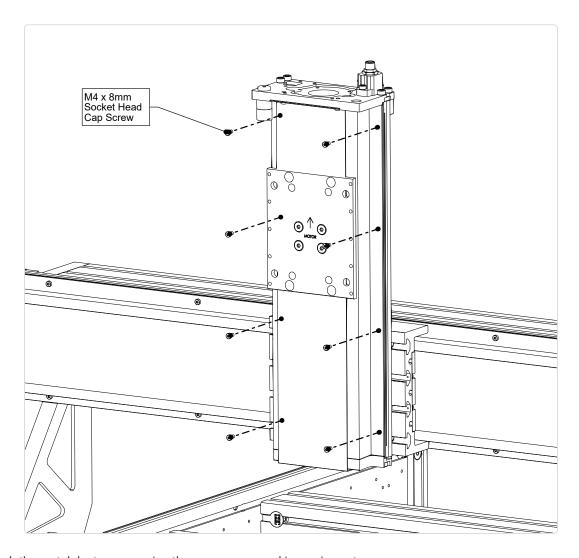
• Attach the metal dust covers using the screws removed in previous steps.
