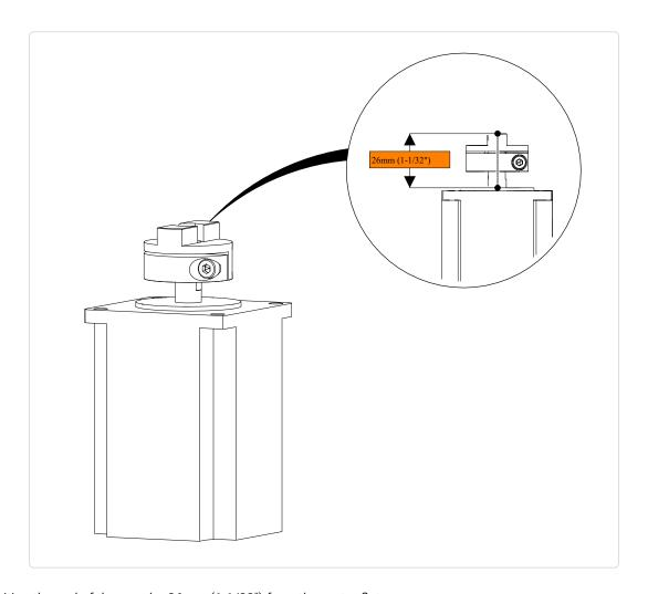
• Position the end of the coupler 26mm (1-1/32") from the motor flat.
