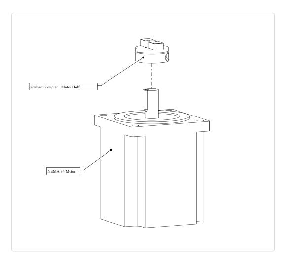
• Slide the motor side of the oldham coupler onto the motor as indicated.
