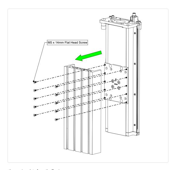
• Remove the moving plate from the Z axis.
