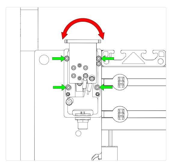
• Loosen the four indicated screws to tram the Tool Height Setter in the x-axis direction.
