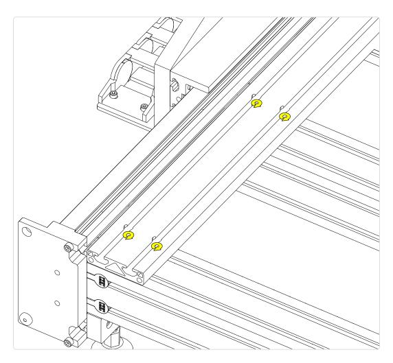
• Partially tighten the tabletop extrusion fasteners.
