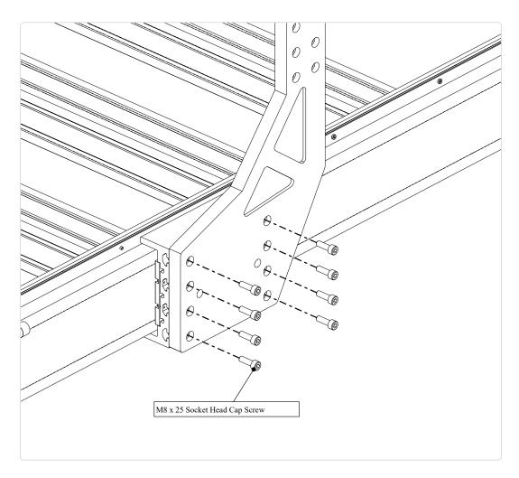
• Thread socket head cap screws into the T-Nuts.
