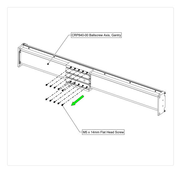
• Remove the indicated screws holding the moving plate to the gantry ballscrew axis.
