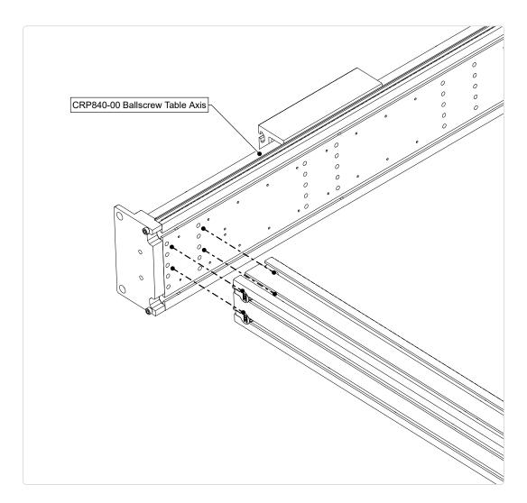
• Thread the screws into the left table ballscrew axis as indicated.
