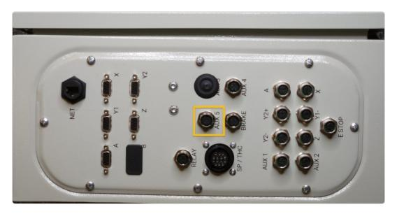
• Connect the existing Ohmic Protection Box sensor cable to the Aux 5 port.
