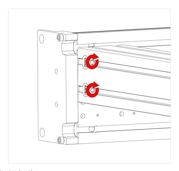
• Tighten the indicated fasteners
