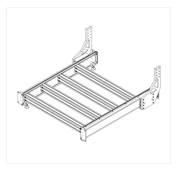
• Slide the risers to the back of the machine.
