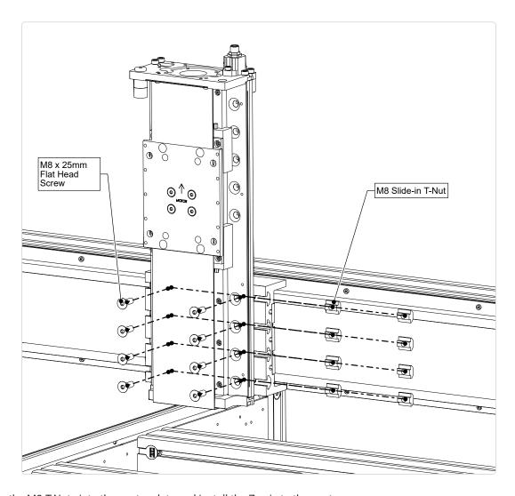
• Slide the M8 T-Nuts into the gantry plate and install the Z-axis to the gantry.
