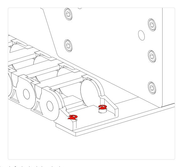
• Tighten the fixed end to the lower bracket.
