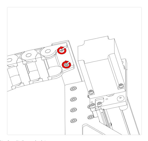
• Tighten the end to the upper bracket.
