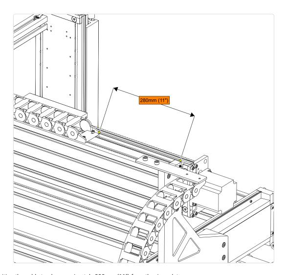
• Position the cable track approximately 280mm (11") from the riser plate.
