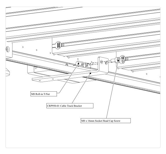
• Install the lower cable track bracket onto the bottom of the base of the machine.
