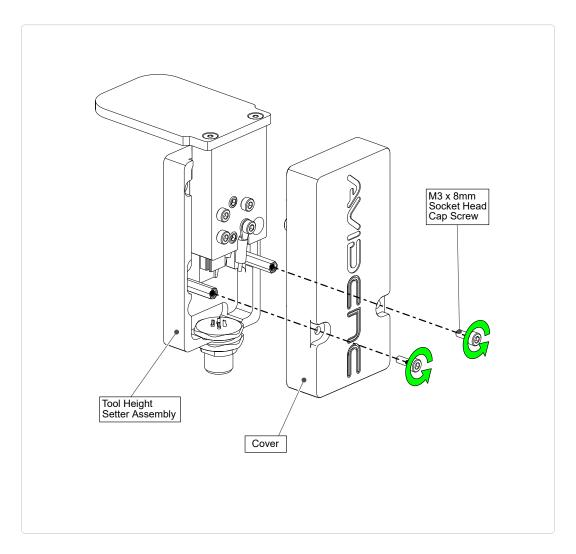
• Remove the Cover from the Tool Height Setter Assembly.
