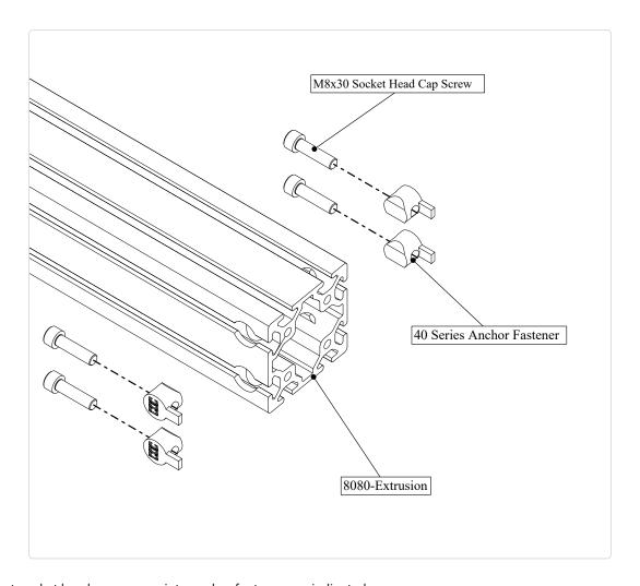
• Insert socket head cap screws into anchor fasteners as indicated.
