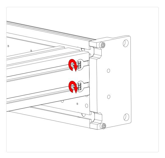
• Tighten all remaining crossmember anchor screws.
