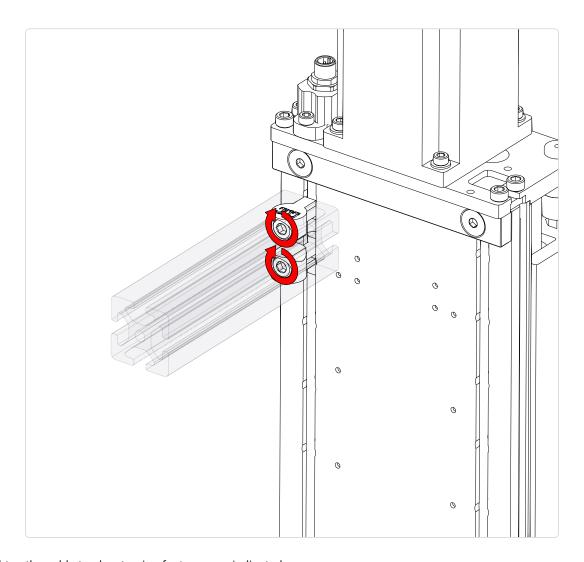
• Tighten the cable track extrusion fasteners as indicated.
