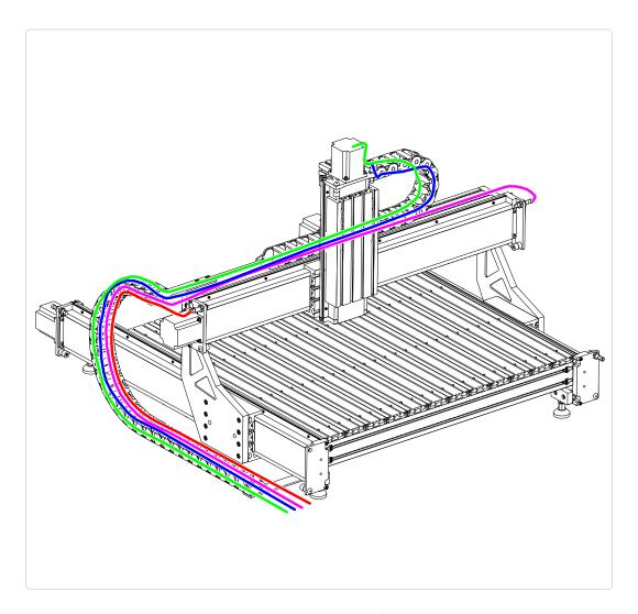
• Route the indicated sensor cables as shown (see table on next page). The remaining three sensor cables can be routed directly to your control box without going through cable track.
