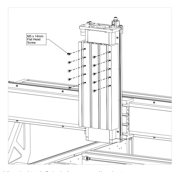
• Attach the moving plate to the Z axis using the screws removed in previous steps.
