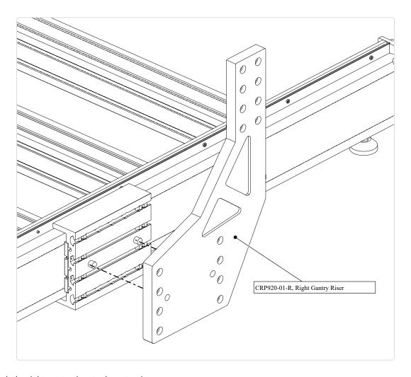
• Attach the right gantry riser to the extrusion.
