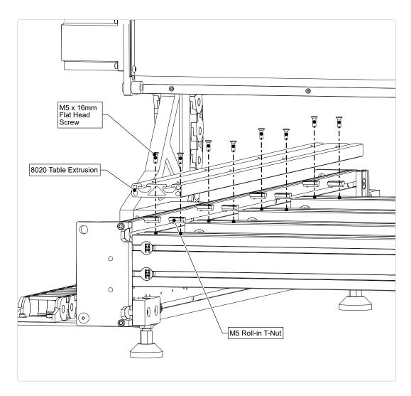
• Attach a piece of tabletop extrusion to the machine crossmembers as indicated.
