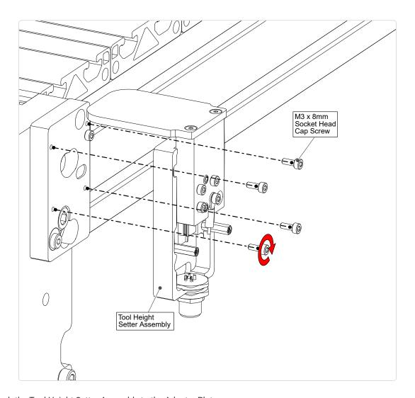
• Attach the Tool Height Setter Assembly to the Adapter Plate.
