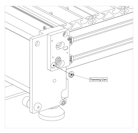
• Insert the Tramming Cam into the pocket on the Adapter Plate.
