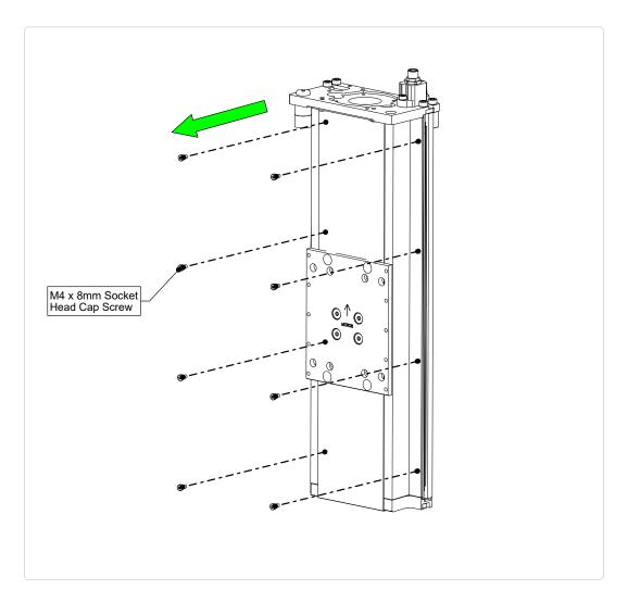
• Remove the metal dust cover screws from the Z axis and set them aside.
