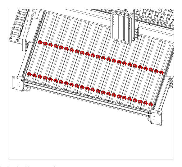
• Fully tighten the tabletop extrusion fasteners.
