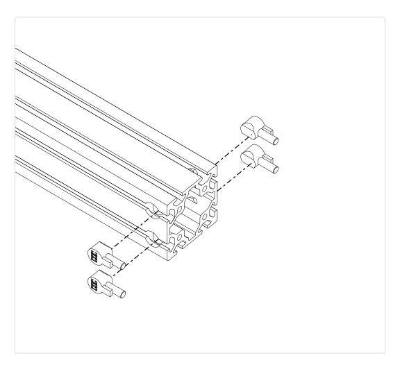
• Slide the anchor fasteners and screws into the extrusion counterbores.
