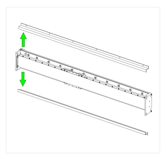
• Remove the metal dust covers from the gantry axis.
