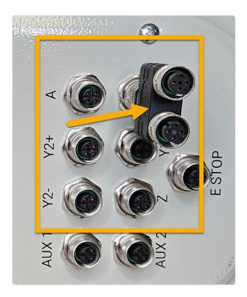
• Install the M12 splitter in the port labeled "X" on your controller.
