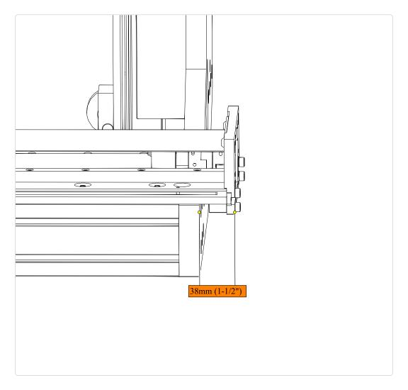
• Position the axis so the motor mount plate is 38mm (1-1/2") from the riser.
