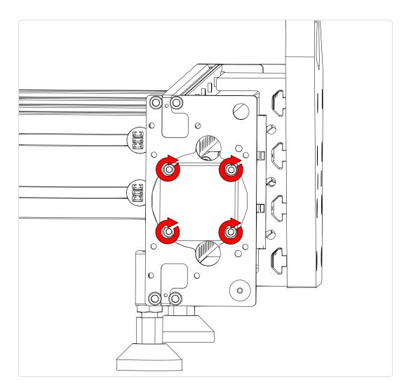
• Tighten the indicated fasteners.
