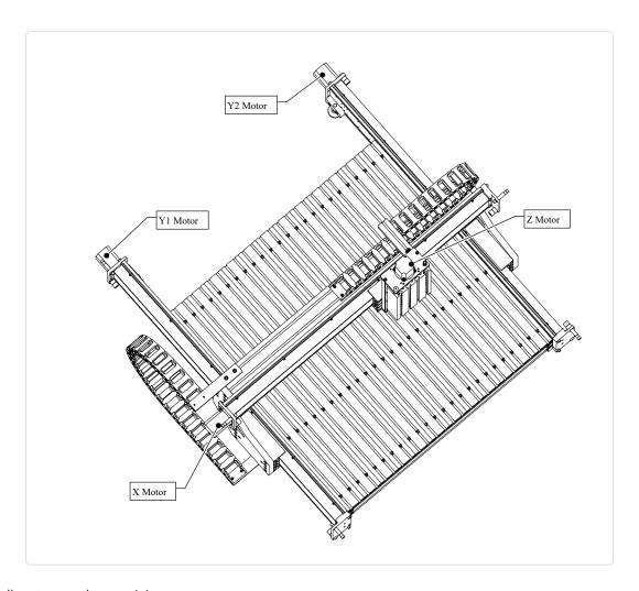
• Install motors on the remaining axes.
