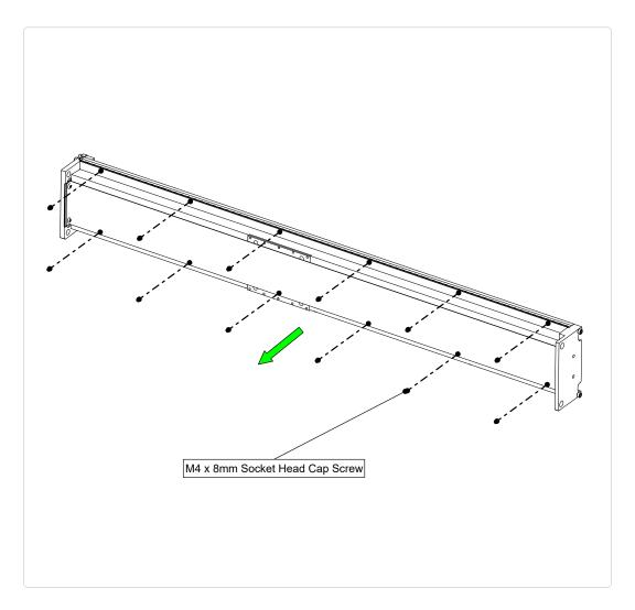
• Remove the metal dust cover screws from the gantry axis and set them aside.
