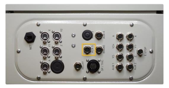
• Connect the existing Ohmic Protection Box sensor cable to the Aux 5 port.
