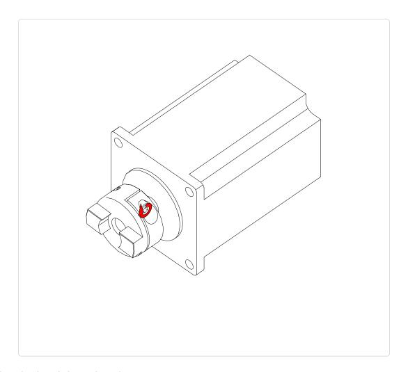
• Tighten the clamp bolt as indicated.
