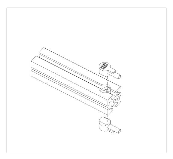
• Slide the anchors into the cable track extrusion as indicated.
