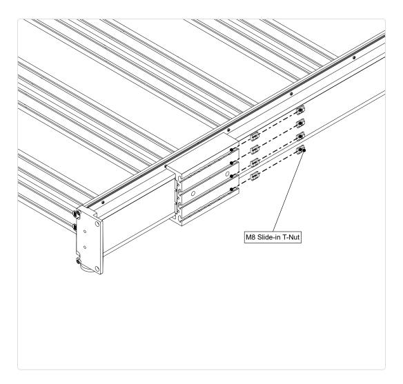
• Slide slide-in T-Nuts onto the right table axis as indicated.
