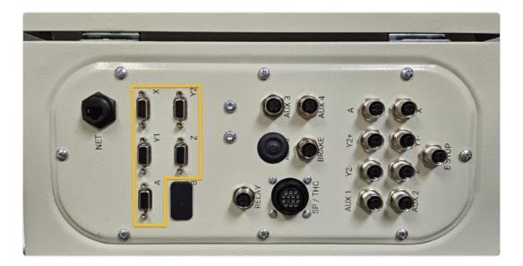
• Connect each motor cable to the appropriate motor port.
