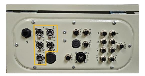
• Connect each motor cable to the appropriate motor port.
