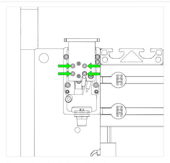
• Loosen the screws noted to tram the Tool Height Setter in the y-axis direction.
