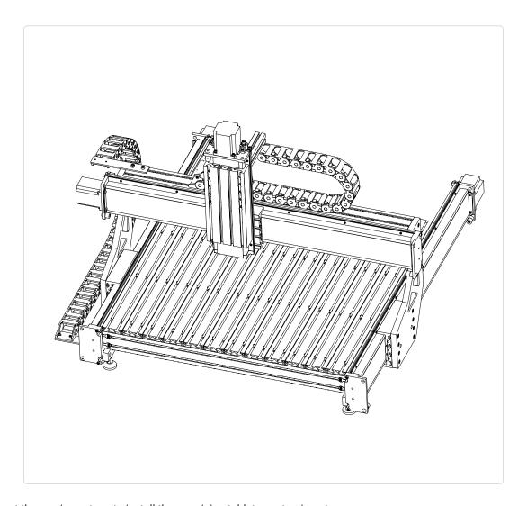
• Repeat the previous steps to install the remaining tabletop extrusion pieces.
