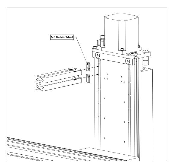
• Attach the cable track extrusion to the Z axis indicated.
