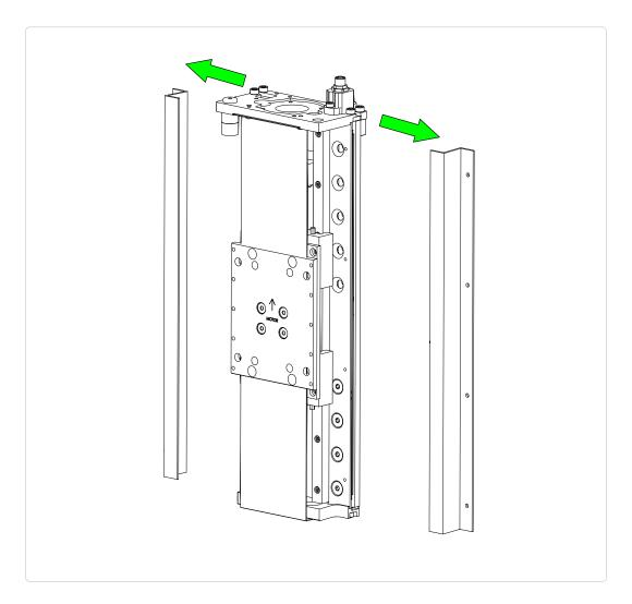
• Remove the metal dust covers from the Z-Axis.
