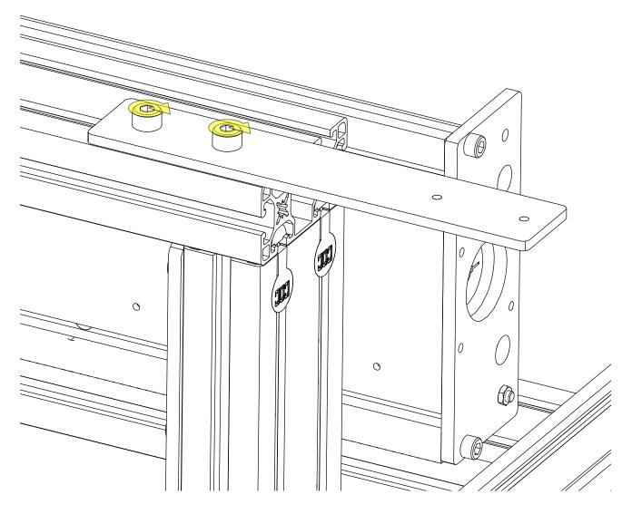
• Partially tighten the highlighted fasteners.
