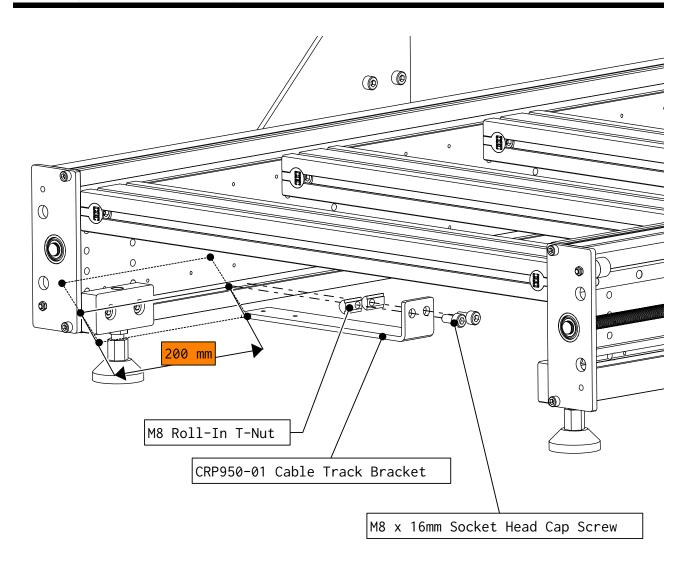
• Attach the CRP950-01 Cable Track Bracket to the machine table approximately 200 mm (7.85") from the bearing plate as indicated.
