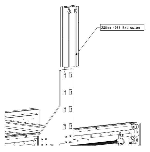
• Slide a 280 mm (11") length of 4080 extrusion onto the riser plate as indicated.
