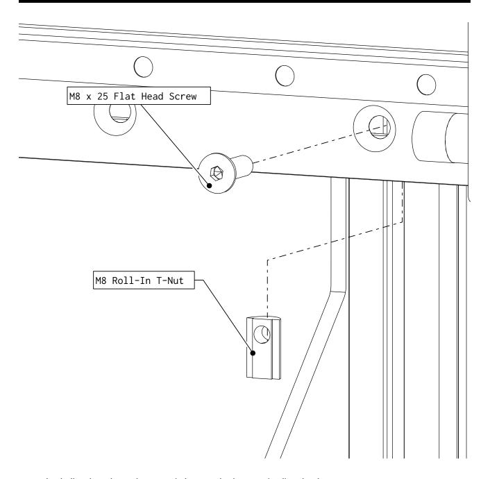
• Install a t-nut and screw into each riser as indicated.
