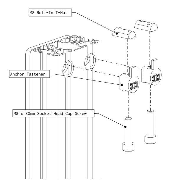
• Slide anchor fasteners, screws, and t-nuts into a piece of riser extrusion as indicated.
