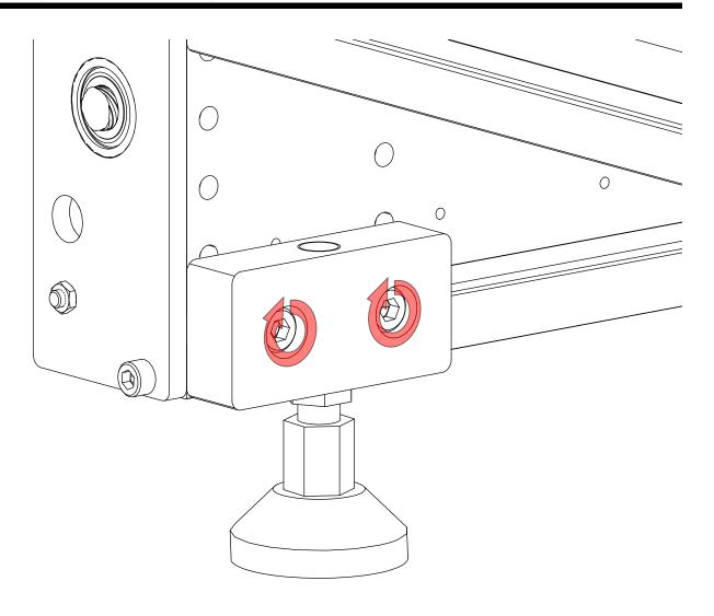
• Tighten the highlighted fasteners.
