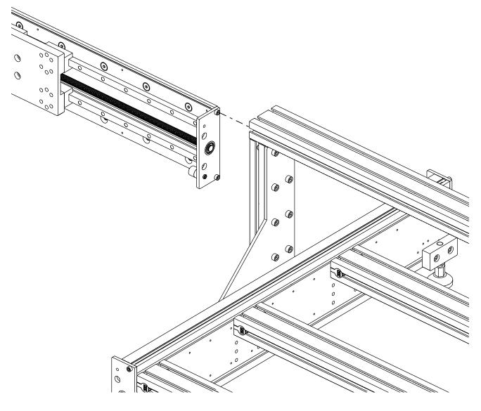
• Slide the axis into the front t-slot of the gantry extrusion as indicated.
