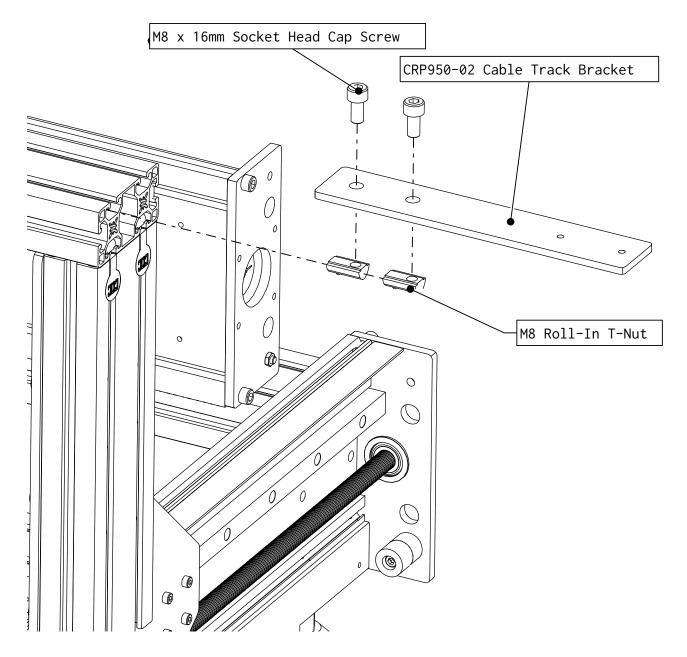
• Thread screws and T-nuts into the CRP950-02 Cable Track Bracket and slide into the gantry extrusion as indicated.
