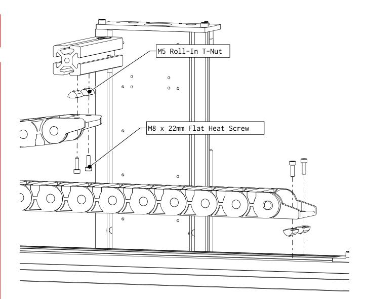
• Install a length of cable track to the cable track bracket and extrusion as indicated.
