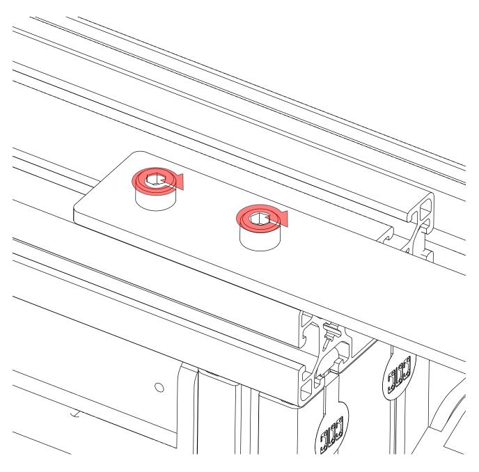
• Fully tighten the highlighted fasteners.
