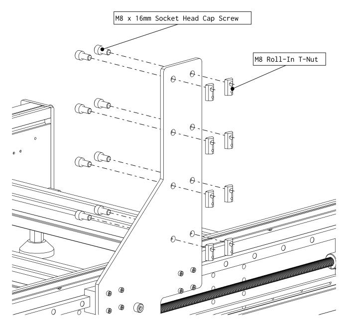
• Thread screws and t-nuts into the riser plate as indicated.
