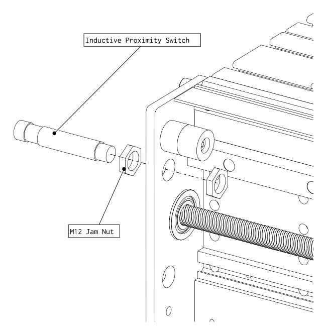
• Install an inductive proximity switch into the end of an axis as inidicated.
