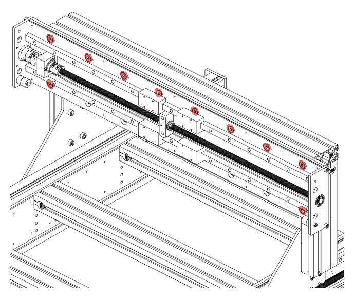
• Tighten the highlighted fasteners.
