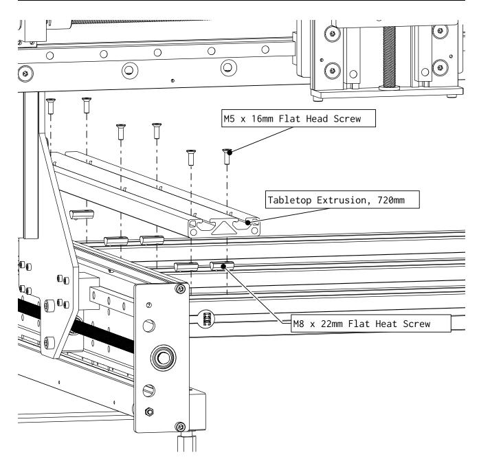
• Install a length of tabletop extrusion onto the machine as indicated.
