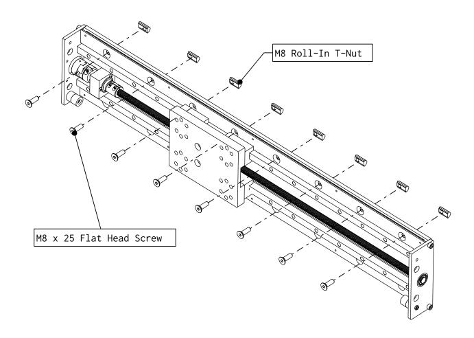
• Thread screws and t-nuts into the Benchtop Gantry Axis.
