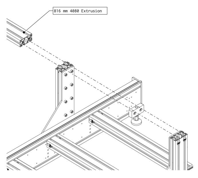
• Slide the 816 mm (32") length of 4080 extrusion onto the previously installed t-nuts as indicated.
