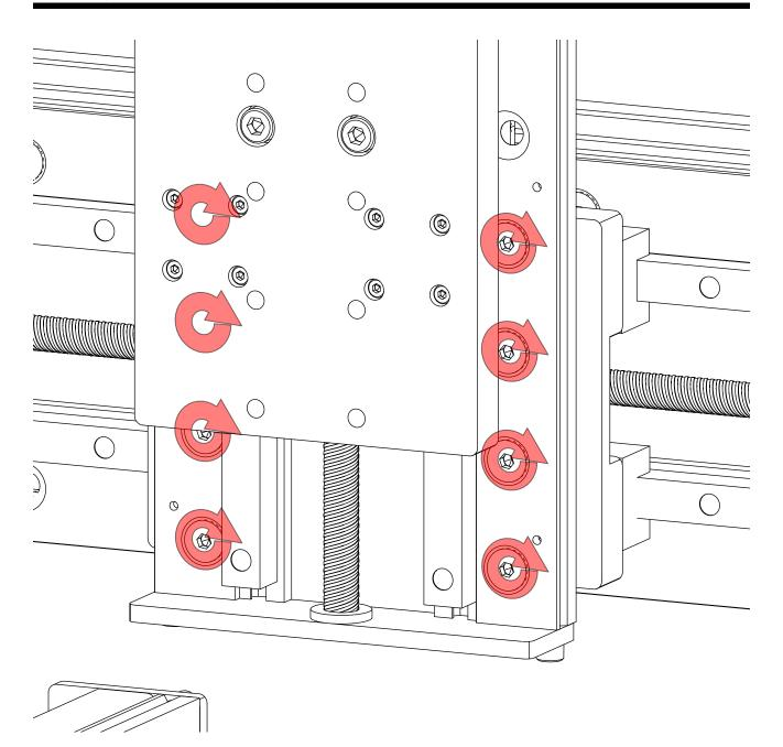
• Tighten the highlighted fasteners.
