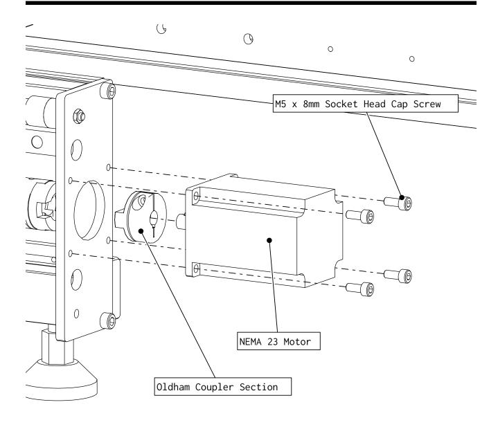
• Install a NEMA 23 motor to the end of an axis as indicated
