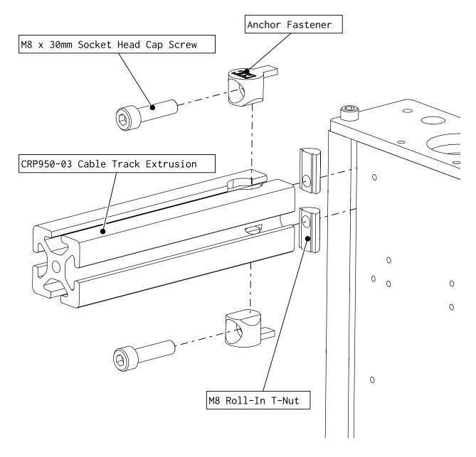
• Attach the CRP950-03 Cable Track Extrusion to the top of the Z-Axis as indicated.
