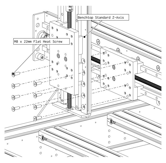
• Attach the Benchtop Standard Z-Axis to the Gantry Plate as indicated.
