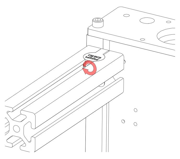
• Tighten both screws in the Cable Track Extrusion anchor fasteners.
