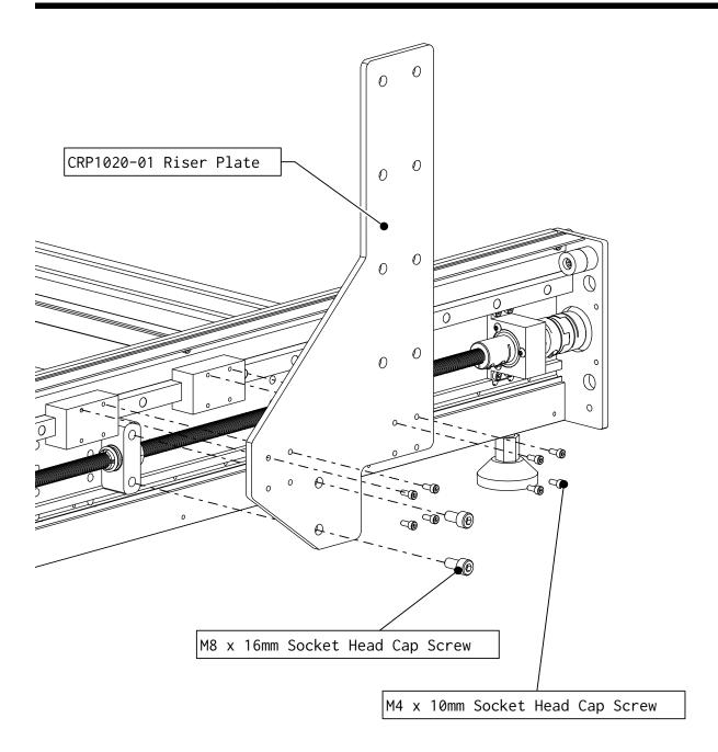
• Attach a Riser Plate to the bearing blocks and acme nut as indicated.
