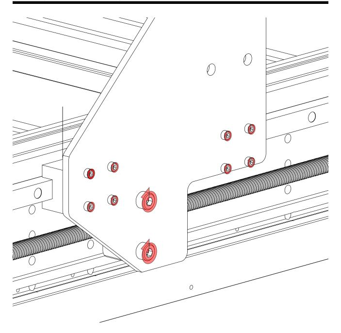
• Tighten the highlighted fasteners.
